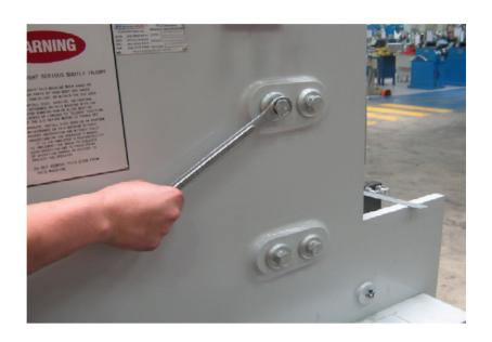
**Step 3.** Set rapid blade adjustment to the correct gap. Repeat operation at opposite end to ensure the blade is parallel.
